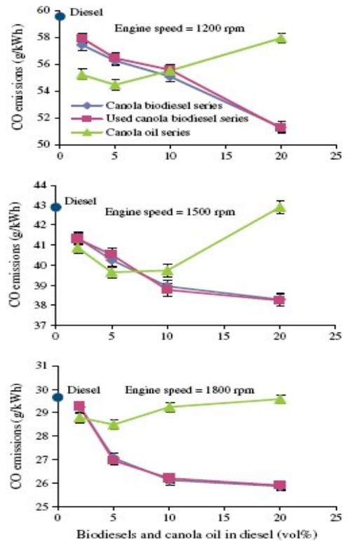
Fig. 5. CO emissions at different engine speeds for various fuels: (a) with engine speed of 1200 rpm, (b) 1500 rpm, and (c) 1800 rpm.
