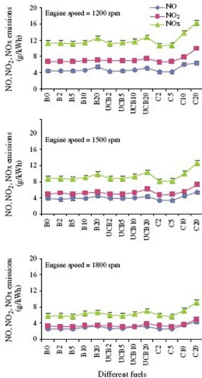
Fig. 4 NOx emissions at different engine speeds for various fuels: (a) with engine speed of 1200 rpm, (b) 1500 rpm, and (c) 1800 rpm.
