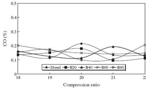
Fig. 6: Variation of carbon monoxide with compression ratio for different biodiesel blends.
