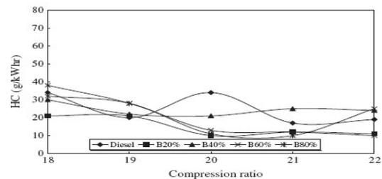
Fig. 10: Variation of HC emission with compression ratio for different blends. Fig. 11. HC emissions at different engine speeds for various fuels: (a) with engine speed of 1200 rpm, (b) 1500 rpm, and (c) 1800 rpm
