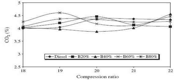
Fig. 8: Variation of CO<sub>2</sub> with compression ratio for different blends.
