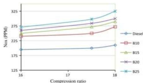
Fig. 1: Variation of NO<sub>x</sub> with the compression ratios for diesel and biodiesel blends at best injection timing (27°).
